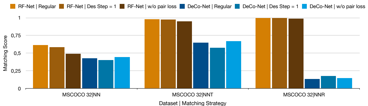
Figure 4.6: Matching scores on MS COCO 2017 with \rho = 32 . RF-Net and DeCo-Net were trained in a regular way (Regular) as described in Section 4.1, with less descriptor steps (Des Step = 1), and without pair loss (w/o pair loss).
