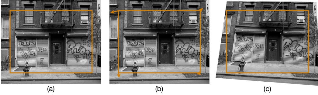
Figure 3.1: Illustration of the data generation pipeline for a low-resolution patch of the synthetic dataset. (a) A crop is taken from an image. (b) The vertices of the crop are randomly perturbed by values within the range [-\rho, \rho] . (c) The four resulting vertex correspondences are used to compute a homography H^{ji} . The inverse of this homography H^{ij} = (H^{ji})^{-1} is applied to the image and a crop is taken from the same position as before.
